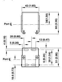
**Neck Mounting** for B72, R72, V72, includes plastic panel nut Use 4 mm (5/32") screws to mount bracket to wall.
