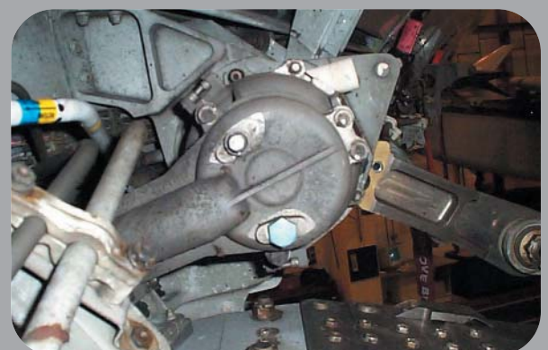
A320 Flap Operating System Rotary Actuator & Offset Gearbox
